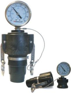
The Edson vacuum gauge is a tool designed to help diagnose problems in a typical pump out system. A pump out system is composed of three major components the pump, controls and plumbing. Most plumbing and pump issues can be found with some simple tests described below.
