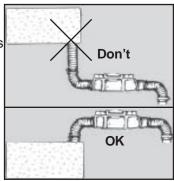
DISCHARGE FITTINGS, PIPE AND HOSE SHOULD ALL BE THE SAME SIZE AND NEVER BE SMALLER THAN THE INLET.
