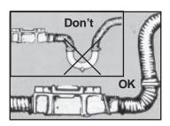
SHOULD NOT INSTALL PUMP WITH POSITIVE HEAD ON THE INLET - Under standard operating guidelines the pump should be above the liquid it is being used to transfer.
