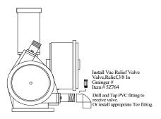
Install the vacuum relief valve in the suction line and adjust to allow a <u>slight</u> flow of air to enter the influent stream.
