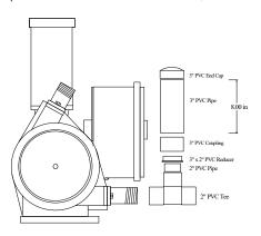
Fabricate and install a chamber in the influent stream (and potentially in the effluent). This creates an air pocket and will act as a "shock absorber" and aid to equalize flow.
