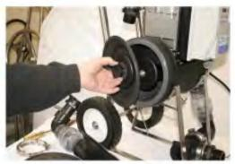
**Rule 2.** Before installing the new diaphragm, run the pump to center the piston in the fully withdrawn position back into the pump frame.
