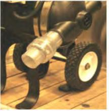
Step 4. Screw the check valve, sealing washer and 1 1/2" close nipple into the pump base after coating the close nipple threads with a light coating of a non-petroleum based, teflon grease. By hand, tighten the valve to the pump base until the sealing washer is pressed tight between the two surfaces. Using a pipe wrench if necessary, continue to screw in the new valve until the flapper hinge is at the top.
