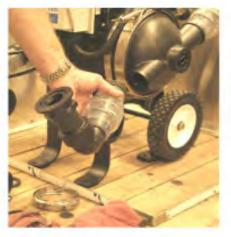
Step 3. Unscrew the check valve-flange elbow assembly(ies) from the pump base(s). If the sealing washer and 1 1/2" close nipple remains in the pump base, leave it. If it comes off with the check valve, it and the flange elbow must be removed from the check valve being replaced. They will be used with the new check valve.
