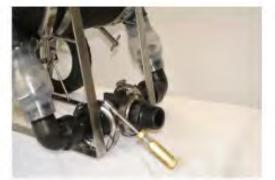
Step 1. Remove the 2" Flange V Clamps and Gaskets on the suction and discharge Tee only on the side of the diaphragm being changed.
