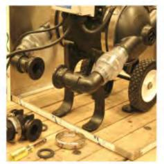
Step 5. Using sealing paste on the threads of the flange elbow, screw it into the check valve. Screw it in until it is aligned with the opposing assembly. Use the flange tee to check the alignment and then go ahead and change the opposing check valve if necessary following the same procedures
