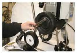
Step 4. Use a 1/2" drive or a cresent wrench to unscrew the diaphragm retaining nut, lower standard and diaphragm from the piston.
