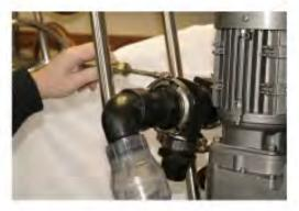
Step 5. Use a little teflon grease to hold the gaskets in place while you align the Pump Base & Valves Assembly. Hold the Pump Base tight to the diaphragm with your body while you fit and tighten the large pump base V Clamp. Re-install the 2" Flange V Clamps on the suction and discharge Tee before starting to change the other diaphragm.
